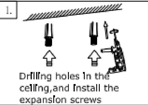
Drilling holes in the ceiling, and install the expansion screws
